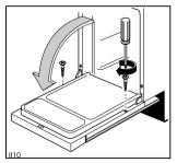
Once the correct position has been found, open the door and fasten the decor panel on the lower section by means of the two long 4x40 screws provided, using the holes through the inner door (see fig.).
